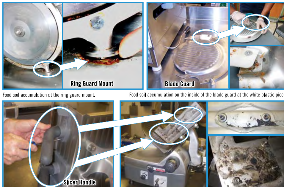
Surfaces under the slicer handle can accumulate food soil and debris and require monitoring to prevent build-up.
